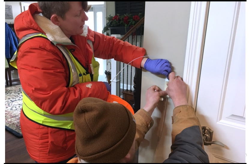
Tubing affixed to selected sampling location with masking tape
