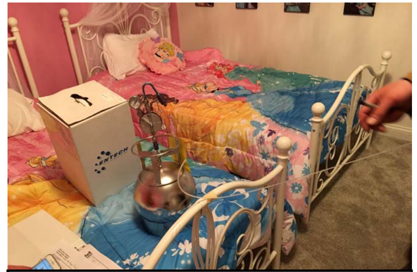
Co-located Summa can and tubing (run to continuous monitor) in child's room
