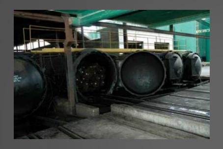
Wood is pressure treated in a retort with a solution of PCP suspended in a petroleum carrier oil.
