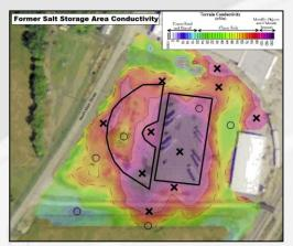
groundwater plume. Surface water was also sampled at multiple locations within the adjacent creek. MUNDELL scientists performed electrical conductivity surveys in the area of the former salt storage pads to identify areas of likely subsurface salt impacts. Initial subsurface soil and groundwater grab samples confirmed the areas of elevated chloride concentrations corresponding to the conductivity survey.
