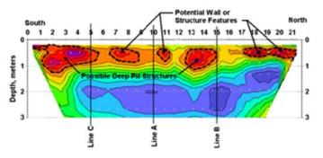
changes in the shallow material properties observed in the ground penetrating radar profile lines. A pueblo with connecting rooms, several deep storage pits, and three burials were identified. Use of multiple geophysical techniques allowed for cross-correlation of anomalous areas, enhancing the likelihood of finding features of significance.
