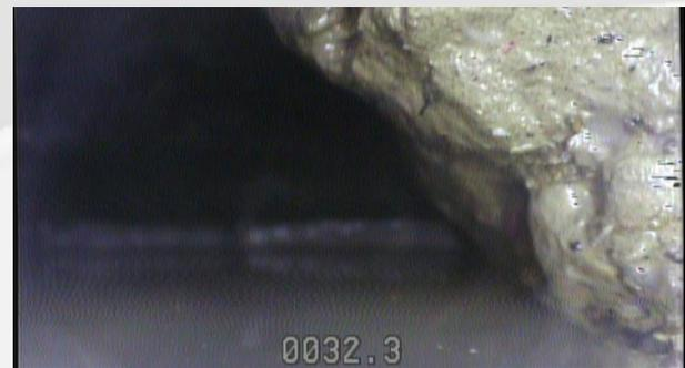
**Figure 1:** A downhole camera image displaying the presence of a subsurface void.
